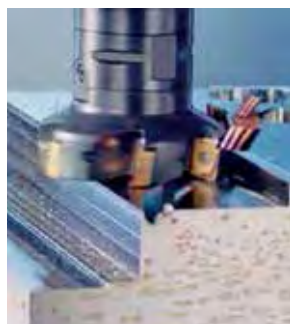
Entry using the 'roll-in' method; wear after 800 machining passes
